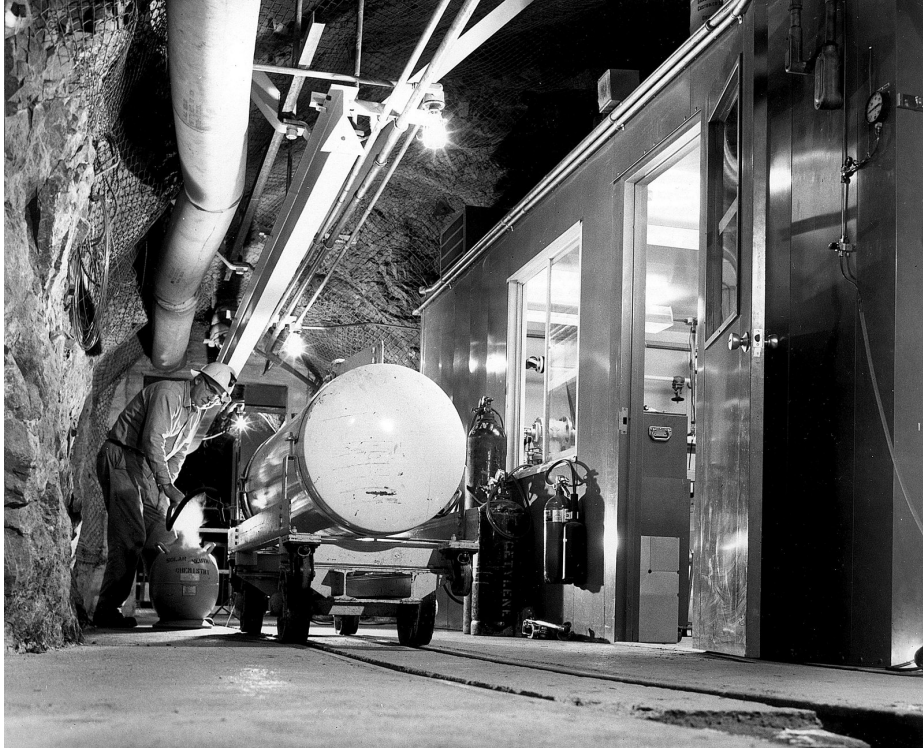
Figure 1.7: Homestake Mine solar-neutrino detector: the large perchloroethylene tank of the Brookhaven / Davis chlorine experiment, photographed underground. Public-domain U.S. Department of Energy photograph (Wikimedia Commons, HD.6B.411).
